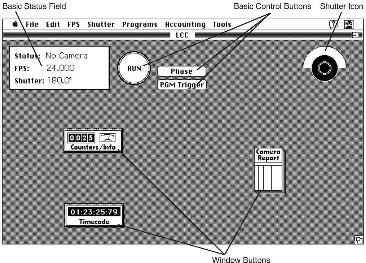
The Main Screen allows the user to read the status of the camera and to control its features. Clicking on one of the *Window Buttons* will open up the respective window.
