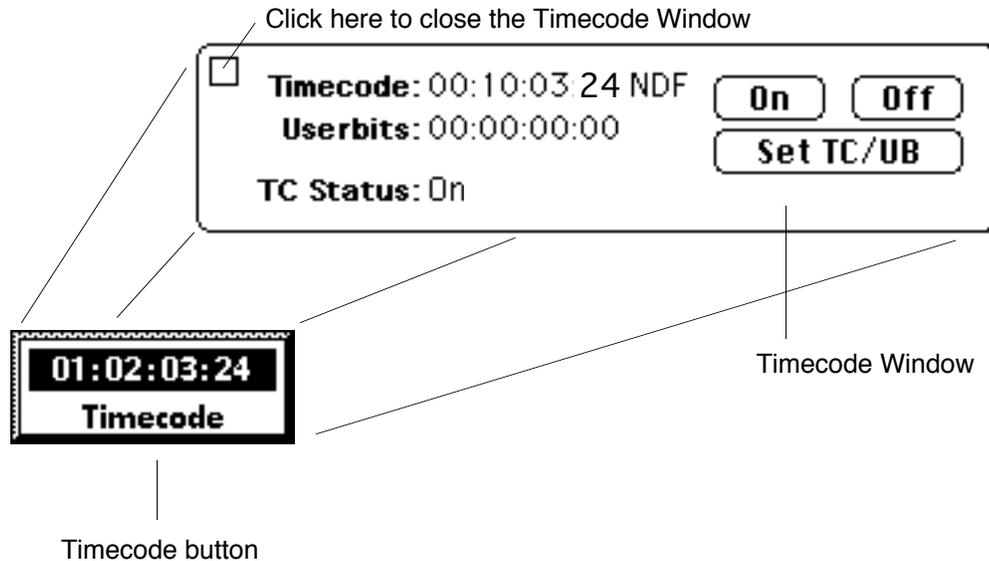
Clicking the *Timecode* button will open up the *Timecode* window. Once opened, this window can be closed by clicking in the square at the top left of the window.
