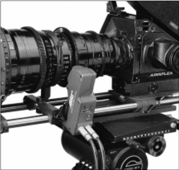
Motor unit CLM-1 mounted on the ARRIFLEX 35 III
